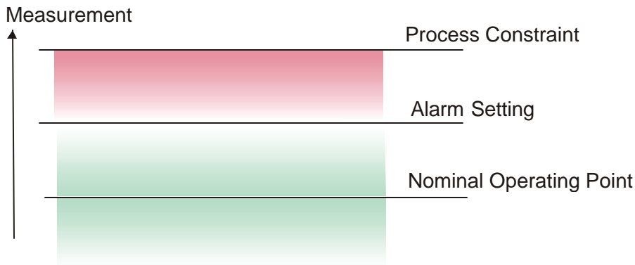
Figure 5.2a: The process has a suitable gap between the normal operating region and the buffer required to correct the process before an actual process constraint is hit.
